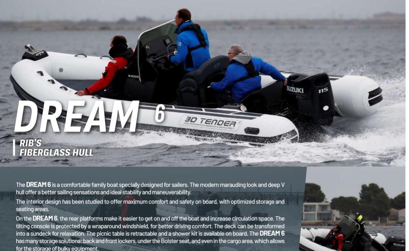
The tubes are available in heat-welded Valmex® PVC from the German company Melher or in HYPALON ORCA® fabric
